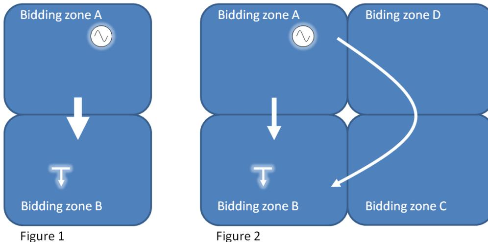
In figure 1, the bidding zones A and B are interconnected in a radial way. Just like the Danish-German AC border, there is a one-to-one translation from the scheduled power exchange between those bidding zones into a physical cross-border flow on the lines. Translated into the flow-based parameters, this means the interconnection has a PTDF = 1. With the general flow-based equation being:
